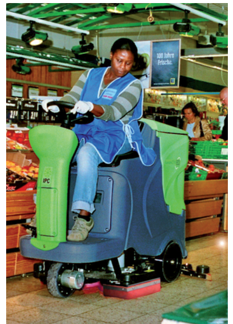
Micro fibre pads (600 g/m - 0,35 lt/min)
